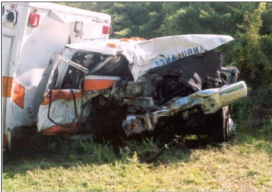
Photo 5. Damage to driver's cab.
