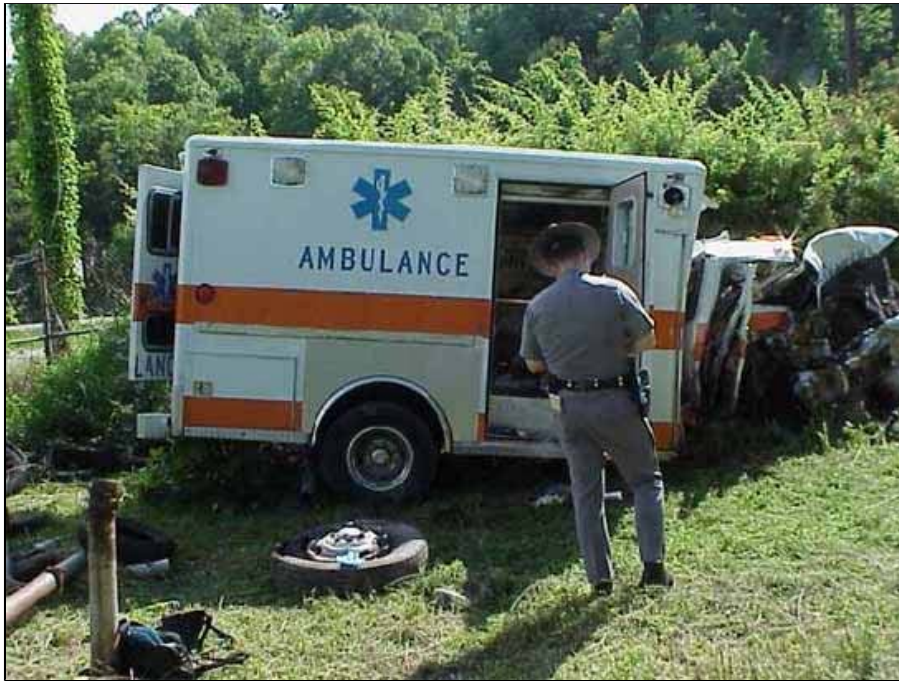
Photo 4. Driver's cab and patient compartment. Note minimal damage to compartment.
