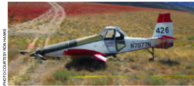
This single-engine airtanker (SEAT) crashed in Nevada during an initial-attack drop in high winds. This crash is an example of “controlled flight into terrain” (CFIT), which occurs when an airworthy aircraft is flown into terrain with inadequate pilot awareness of the impending collision. CFIT accounts for approximately 43 percent of all USFS airtanker accidents.
