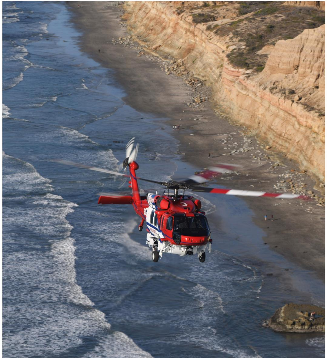
*With a full load of fresh water, the Firehawk helicopter can reach speeds of 140 mph (125 knots) on its return to the fire line.*
