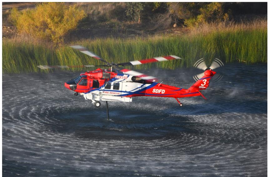
*The S-70i Firehawk helicopter hovers 10 feet above a water source to refill the 1,000-gallon external tank in just 45 seconds.*
