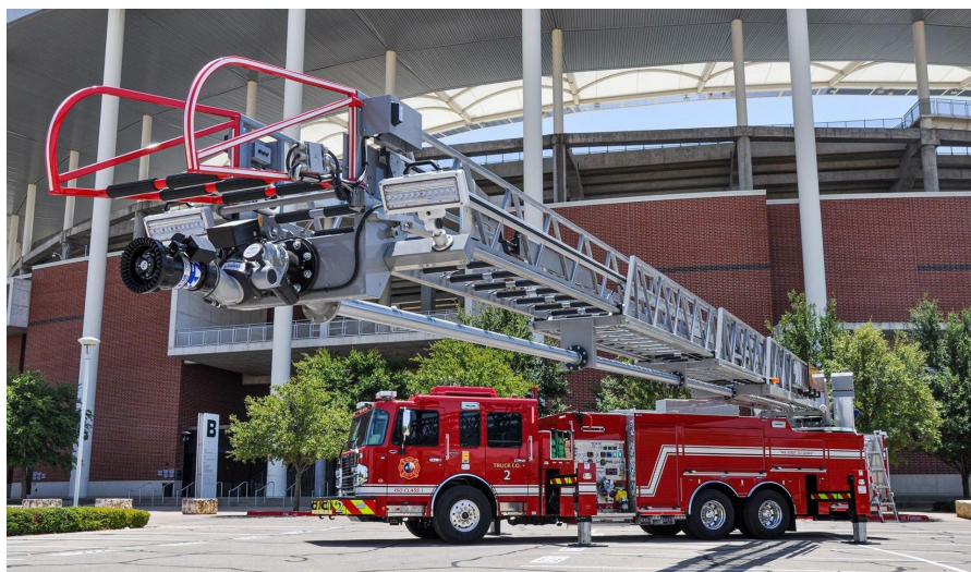
Custom Waco Fire Department (TX) Quint 105-foot aerial, 400-gallon tank, 1,500 GPM pump
