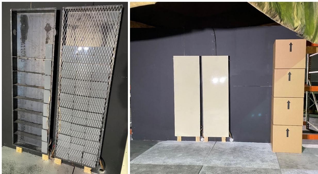
Figure 190 – Interior of ESS units (left) and complete test setup (right) for Scenario 1.
