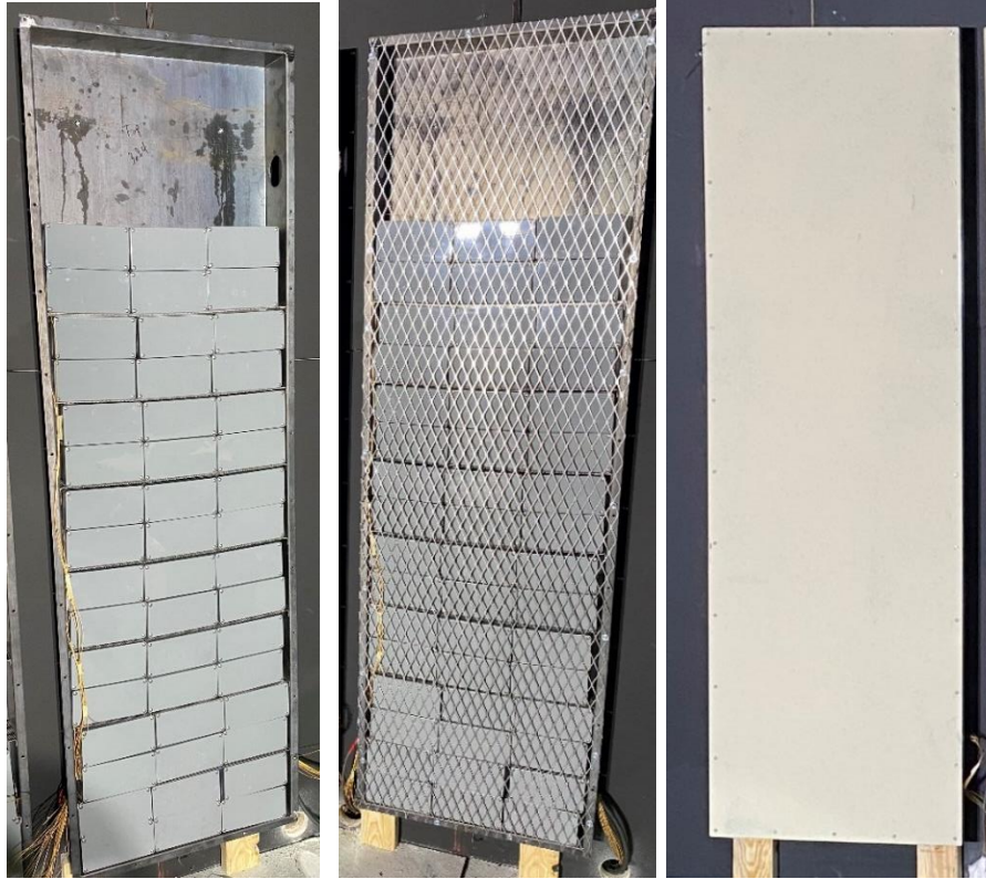
Figure 33 – Unit construction with modules (left), expanded metal insert layer (center), and sheet steel cover (right).
