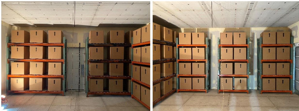
Figure 34 – Rack storage of commodity along C-side wall (left) and D-side wall (right). For Test 2 – 4, the center rack on the D-side wall was replaced with residential ESS units.
