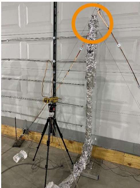
Figure 47 – Heat flux gauge placement (outlined in orange).
