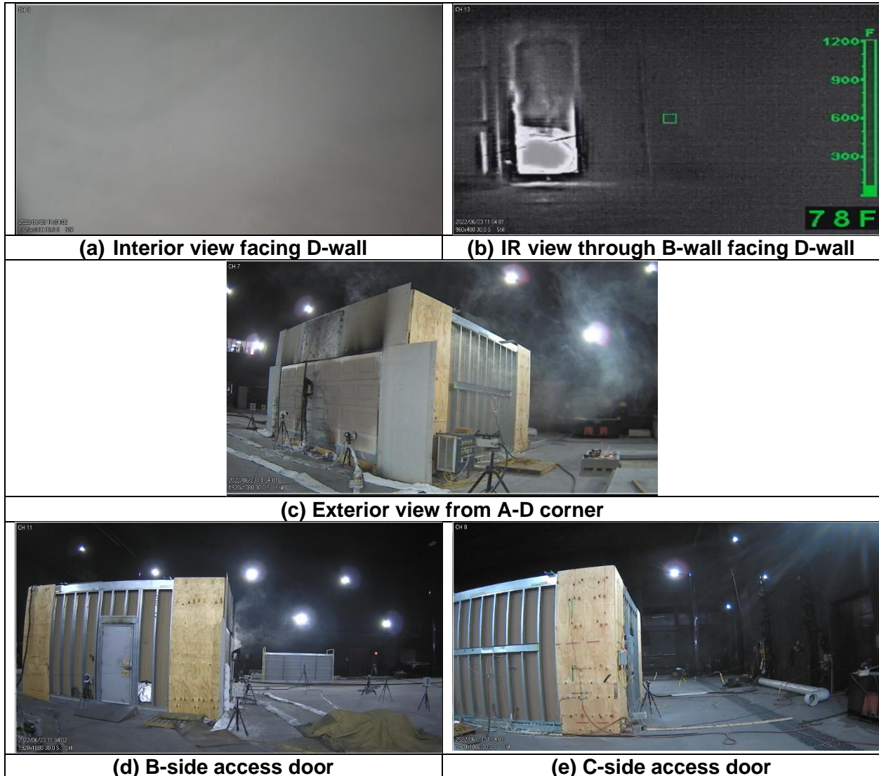
Figure 107 – Exterior view during propagating thermal runaway (30:50, TR + 10:20).
