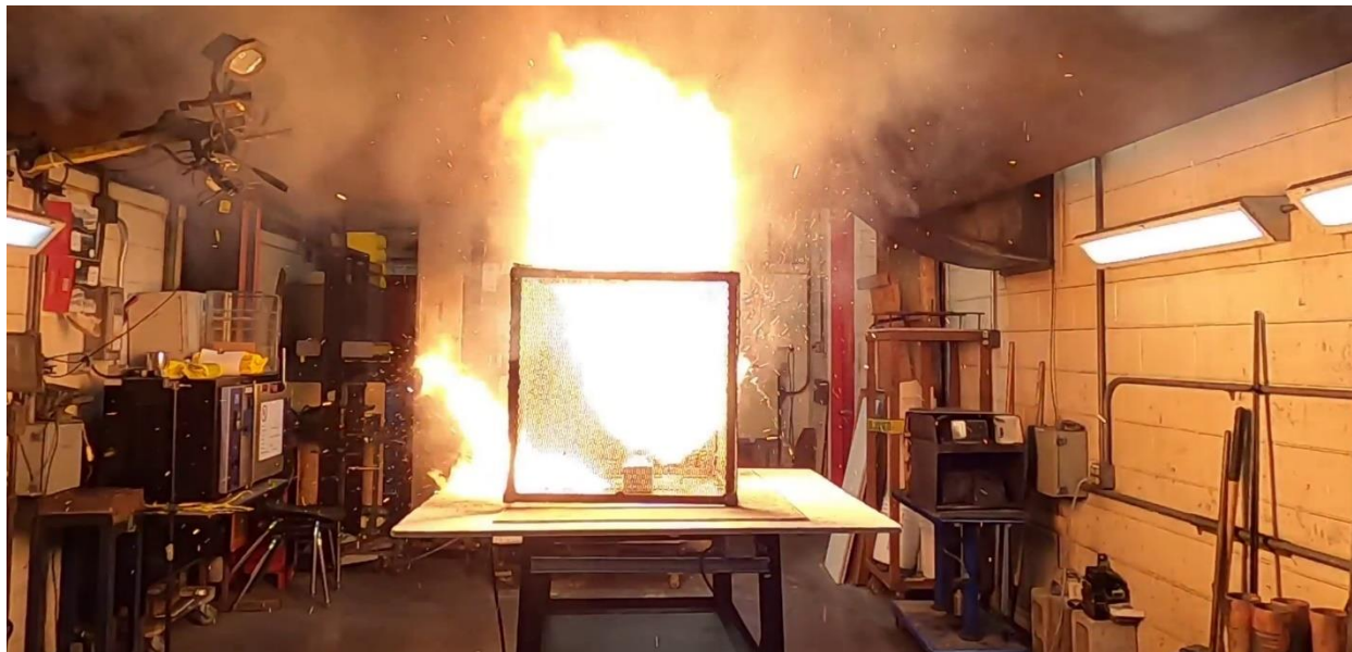
Figure 189 – Photo of module at peak heat release rate.
