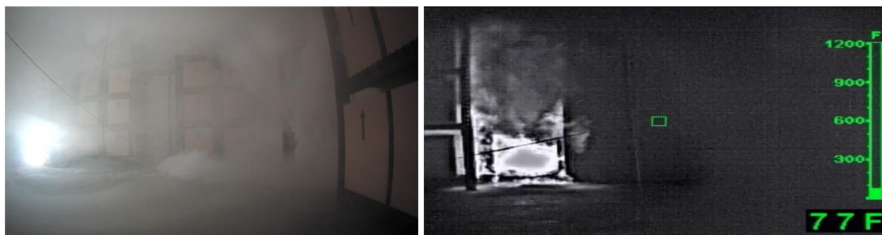
Figure 84 – Gas release and heat development in ESS unit enclosure at 29:43 (TR + 09:13).
