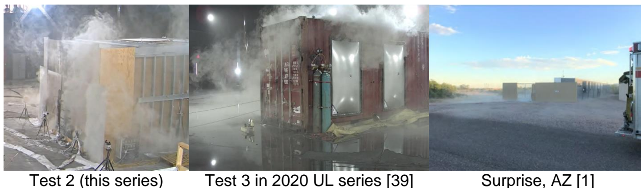
Figure 185 – Sequence of images from different instances of accumulated battery gas leaking from structures.
