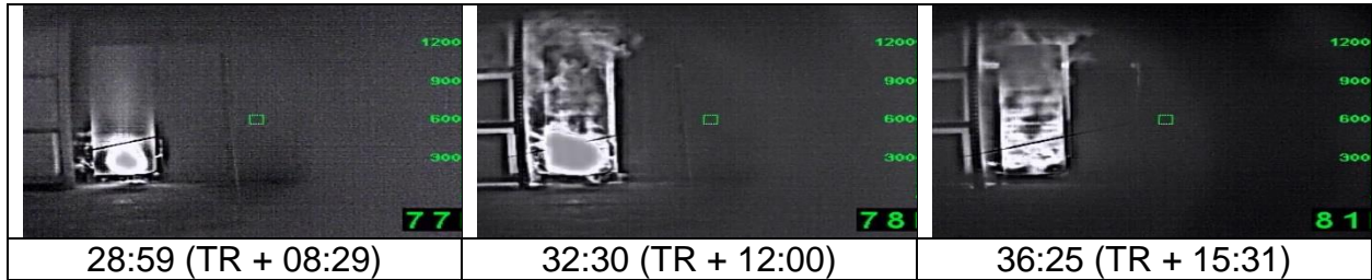
Figure 91 – Thermal images of thermal runaway propagation through Unit 1 in Test 1
