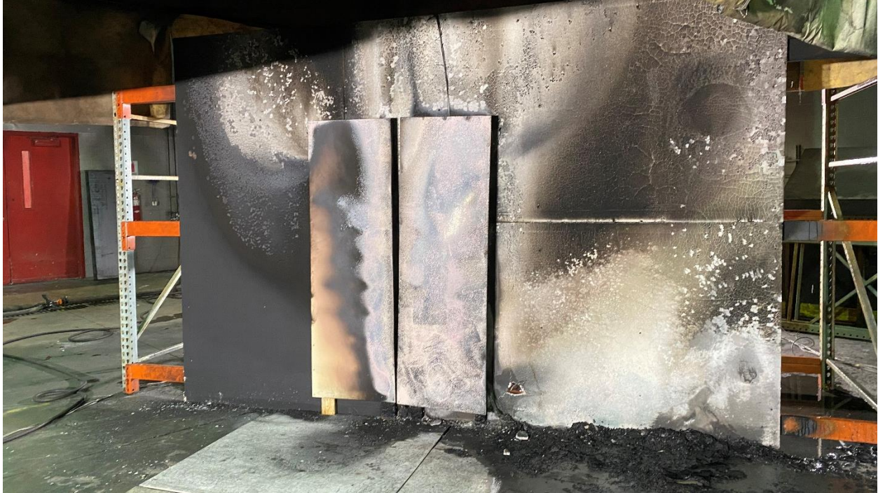
Figure 195 – Post-test condition of ESS units and Commodity boxes in Scenario 1.
