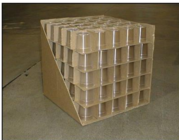
Figure 35 – Cut away of single box showing cups.
