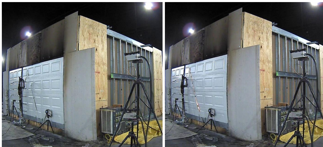
Figure 165 – Exterior effects of deflagration (Left – Initial, Right – Peak deflection) in Test 4.
