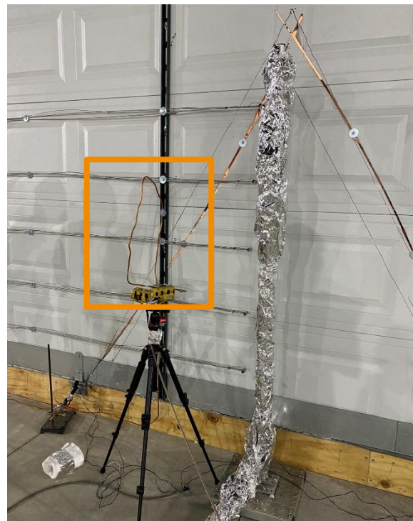
Figure 42 – Location of gas probe in front of garage door (outlined in orange, sampling location near bottom of rectangle).
