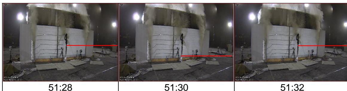
Figure 139 – Short lived transient pressure increase affecting neutral plane height.
