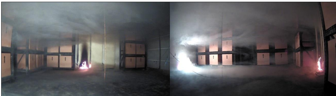
Figure 186 – Visual indication of thermal runaways in Test 4: hot gas layer developing at ceiling and a clearly defined smoke layer remains at the floor.
