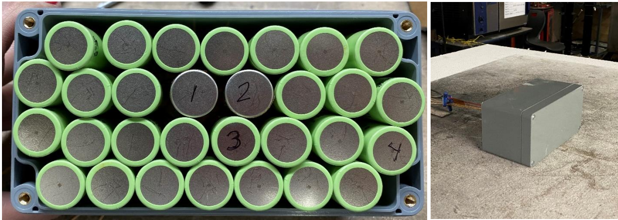
Figure 187 – Module construction (left) and assembly (right).
