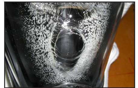
Typical fire-fighter breathing apparatus damaged in NIST tests shows facepiece warping under high heats.
